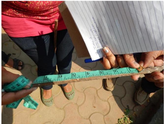
*An iron rod was hammered into the soil around the tree base ensuring no damage to the roots, to find out the depth of the soil in the box below the tree base. The soil layer was found to be only 8 inches deep*
